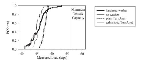
*Fig. 5. Cumulative density function of loads required to close half of the gaps,* %-in. A325 bolts (minimum pretension is 39 kips and minimum tensile strength is 56 kips).
