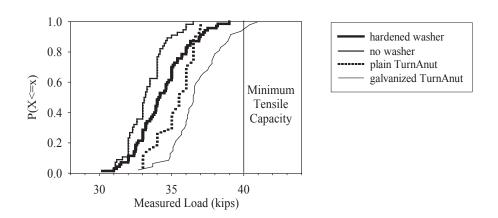
Fig. 4. Cumulative density function of loads required to close half of the gaps, <sup>3</sup>/<sub>4</sub>-in.-diameter A325 bolts (minimum pretension is 28 kips and minimum tensile strength is 40 kips).
