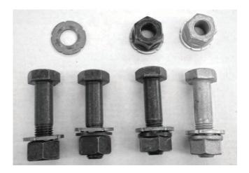
Fig 2. Test configurations from left to right; DTI without washer, DTI with washer, plain TurnAnut DTI, galvanized TurnAnut DTI.
